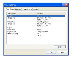
You can click on the [Page Setup], [Finishing], [Paper Source], [Quality], or [Configuration]/[Device Settings] tabs to view a list of printing preferences for each sheet.
